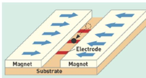
**MOVING EXPERIENCE** Droplet (circle) is levitated magnetically between two fixed magnets and moved by current pulses through electrodes embedded in substrate.
